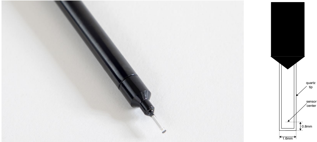
Figure 3: Left: Closeup photograph of the EUAPDDVx probe. Right: dimension of the probe tip and sensor location.
