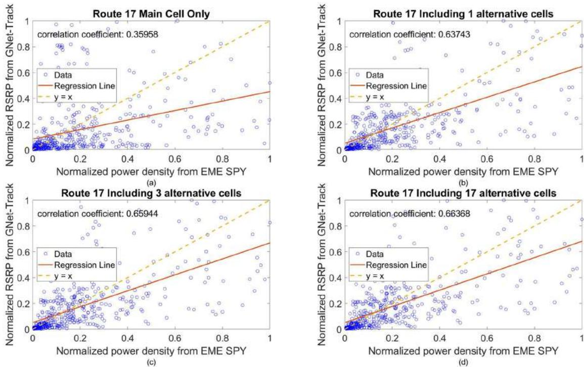
Fig. 5. G - NetTrack Normalized RSRP and EME Spy Evolution normalized power density for Route 17 with a) RSRP: Main Cell Only, b) RSRP: Including 1 alternative Cell, c) RSRP: Including 3 alternative Cells, d) RSRP: Including all 17 alternative Cells.
