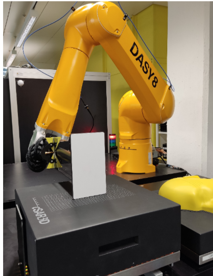
Figure 6: Measurement setup for the study using DASY8 3D [58], using a wooden block to represent the device under test.
